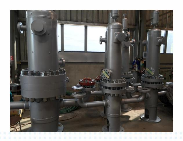
innogy Gas Storage, UGS Štramberk, CZ – Gas Drying Equipment (Gas drying columns, TEG Regeneration Unit, Breed Vapours Combustion Unit)
